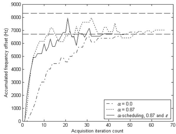
Figure 2. 8-PSK  $\alpha$ -scheduling's faster rise and convergence time
