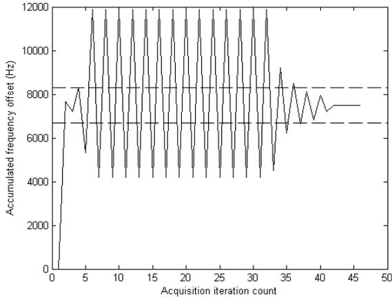
Figure 4. 8-PSK  $\alpha$ -scheduling's convergence time with no noise
