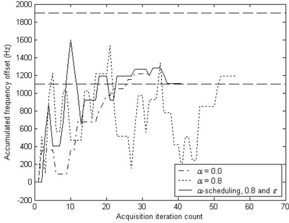
Figure 3. 16-QAM  $\alpha$ -scheduling's faster rise and convergence time
