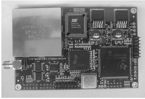
Figure 7. DSP-based low power demodulator
