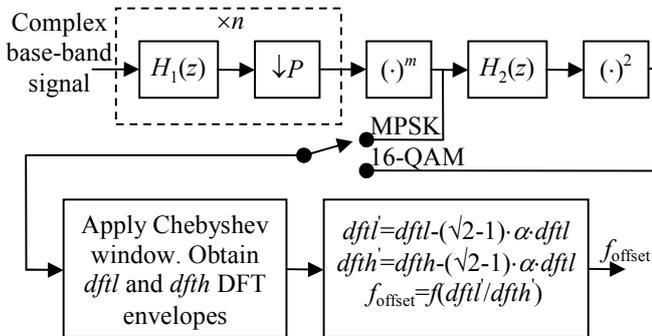
Figure 5. Carrier acquisition section of a high symbol-rate demodulator
