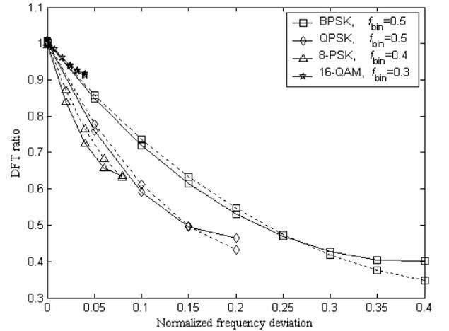
Figure 6. Relationship between frequency offset and DFT ratio, solid and dashed curves correspond to coarse and fine window lengths respectively
