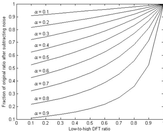
Figure 1. Fraction of DFT ratio computed after noise subtraction as a function of original DFT ratio
