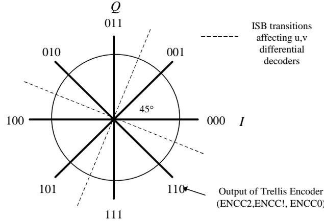
**Figure 2. Symbol mapping to 8-PSK constellation**
