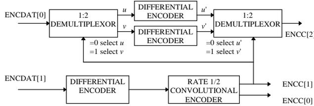
**Figure 1. Phase Ambiguity Encoder for rate 2/3 PTCM using 8-PSK**
