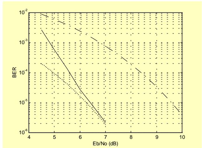
**Figure 6. Rate 2/3, 8-PSK PTCM performance using the simplified branch metric computation (solid line) compared to uncoded QPSK (dashed line). The bound of (3) is the dotted line.**
