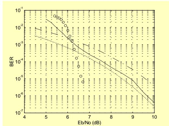
**Figure 9. Rate 5/6, 8-PSK PTM performance (solid line) compared to uncoded QPSK (dashed line). (6) is shown as a dotted line. The circles show the performance with a (225,205) Reed-Solomon outer code over  $GF(2^8)$ .**
