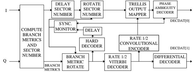
**Figure 3. PTCM Decoder block diagram**
