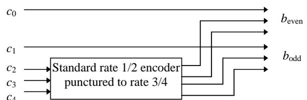
**Figure 7. Rate 5/6 PTCM using a punctured "industry-standard" rate 1/2 code. The odd and even sets of tribits are mapped as in Figure 2.**
